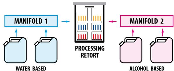
A highly-sensitive ultrasonic reagent sensor (optional) detects the correct solution and its purity while processing. This sensor allows for full specimen safety by detecting any alcohol-based reagents which are exhausted or contaminated by water. Once detected by the sensor, they are not used during the run.
