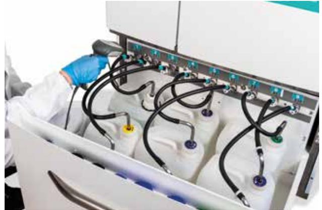
Step 2: reagent loading position scanning
