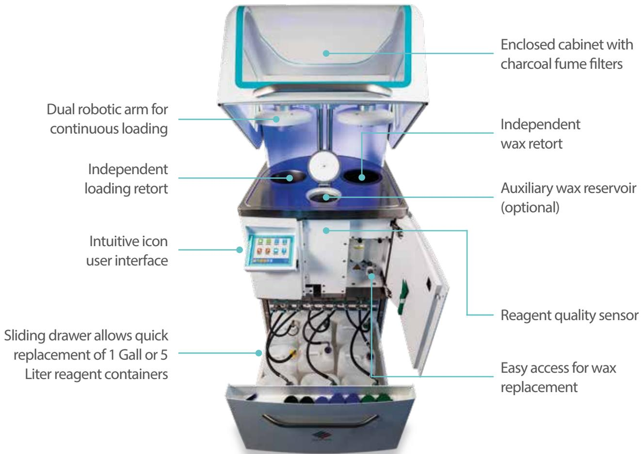
Dual robotic arm for continuous loading
