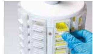
Mold and cassette assembly is inserted in the rack.
