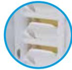
*During the fixation and reagent steps, the molds are angled, so the fluids can flow in and out without retention.*
