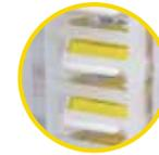
*At the end of wax impregnation (as soon as the rack is lifted) the molds go flat, collecting the necessary paraffin to embed the tissue.*
